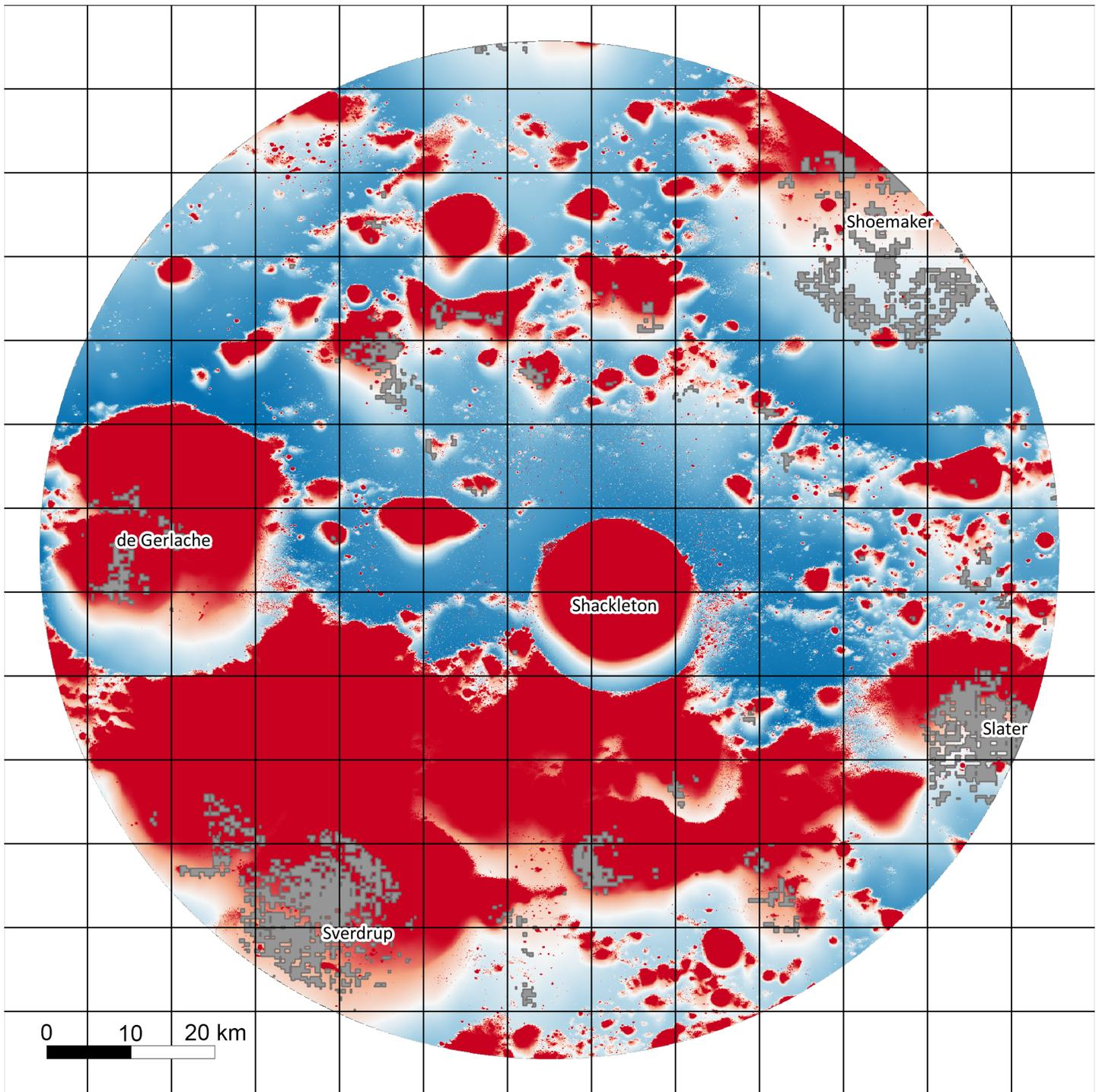
This map shows the average visibility of Earth from the lunar south pole. The Moon is tidally locked, so the same side, called the nearside, faces the Earth. To communicate with Earth, rovers need direct line-of-sight communication with Earth. This map shows the average percent of the Earth is visible with direct line-of-sight communication. Areas that are blue have enough visibility to send data back to Earth. Areas with surface frost are indicated by gray.
