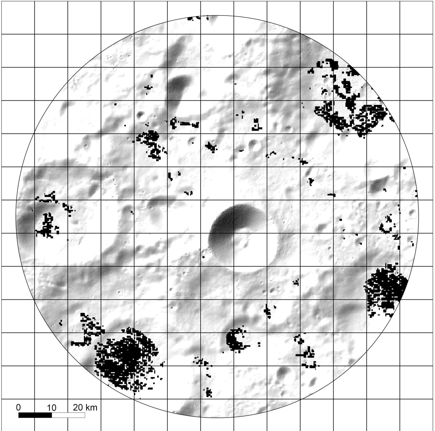
This is the map to print for planning the manned rover mission. It is a hillshade created from a 150 m pixel scale Lunar Orbiter Laser Altimeter (LOLA) digital terrain model (DTM) with the results from the surface-frost analysis overlaid in black.
