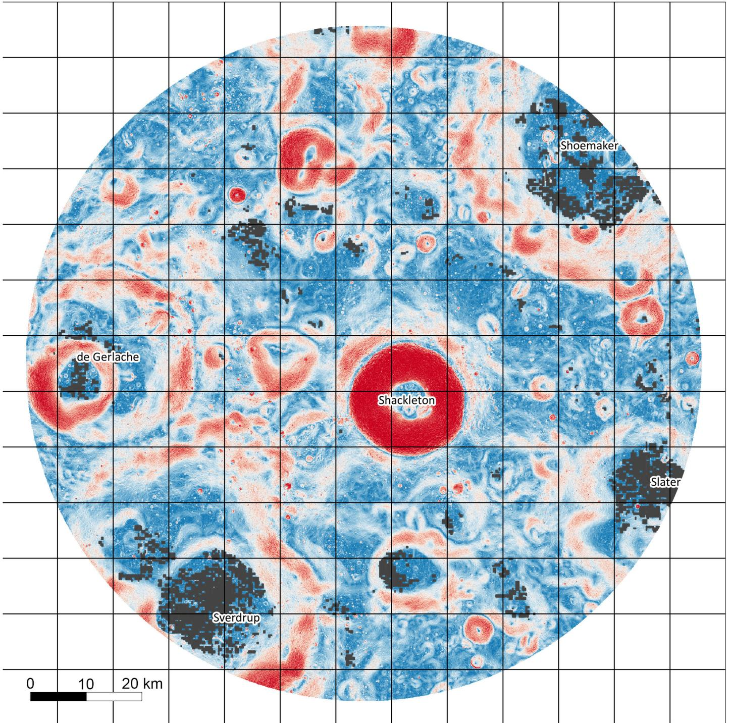
This map shows the angle of the surface, or slope, for the lunar surface. If slopes are 15 degrees or larger the rover cannot traverse them. These are indicated by shades of blue. Landing sites must be even flatter, with slopes  $<5$  degrees (indicated by dark blue). Areas with surface frost are indicated by dark gray.
